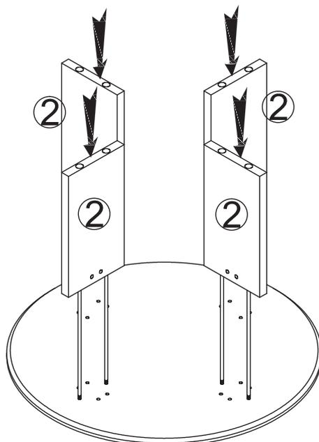
Do not tighten screws until all screws have been assembled !
